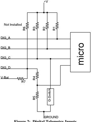
**Figure 2: Digital Telemetry Inputs**
